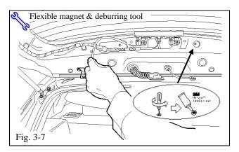
(i) Use a flexible magnet to remove any metal shavings from the inside of the door cavity as well as around the drilling area. Deburr and apply 3M Ultra-Pro Body Sealant to the backdrilled hole (Fig. 3-7).
