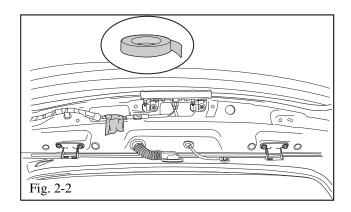
(b) Secure the exposed wire to the outside of the sheet metal with tape (Fig. 2-2).
