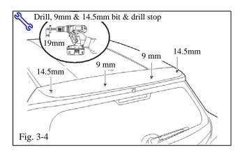
(e) Enlarge each drilled hole to the final sizes as identified on the DIO installation (Fig. 3-4). Make sure that the drill bit is equipped with a drill stop set at 19mm.
